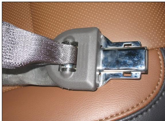
**Figure 13:** Underside view of the inflatable safety belt latch plate within the Ford.
