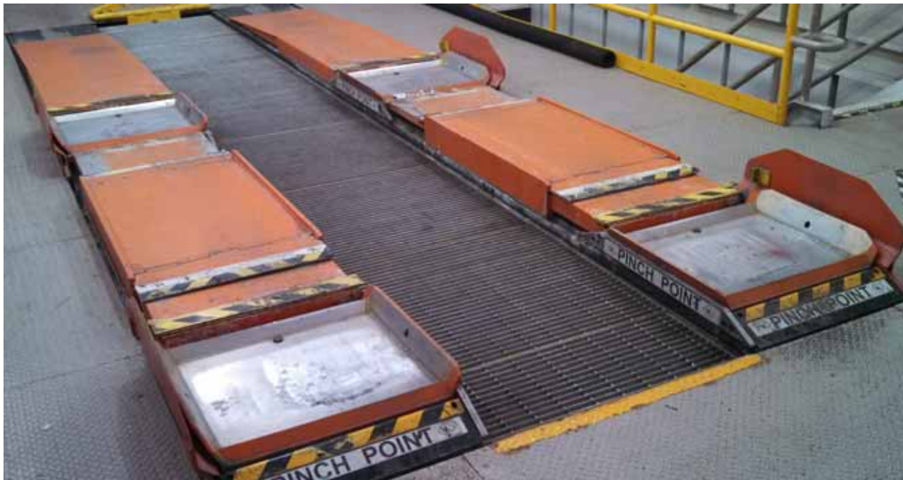
Figure 9A 4 post roadway simulator
