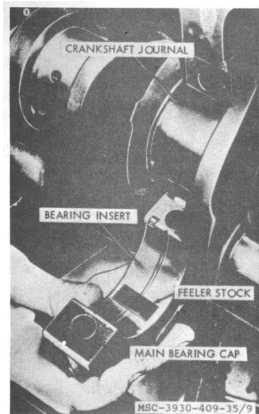
Figure 3-22. Checking main bearing clearances.
