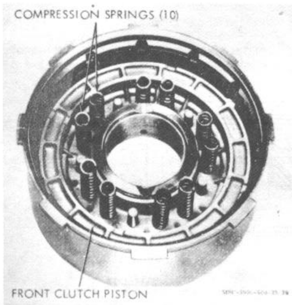
Figure 4-28. Front clutch piston return spring location.
