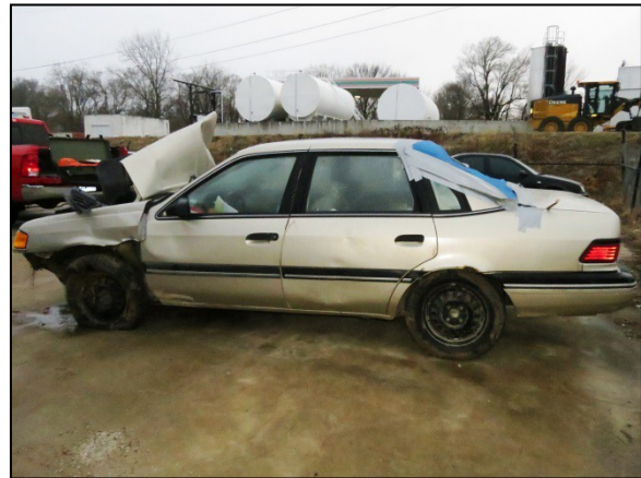
Figure 14: Left plane damage to the Ford.
