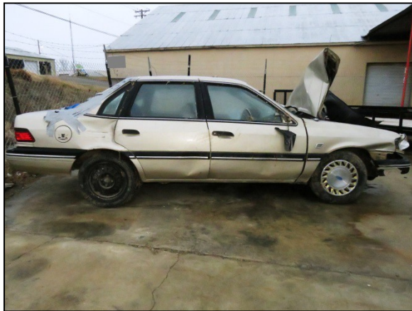
Figure 13: Right plane damage to the Ford.
