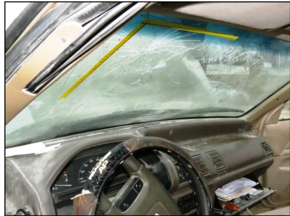
Figure 15: Interior view of the Ford showing driver contact to the windshield.
