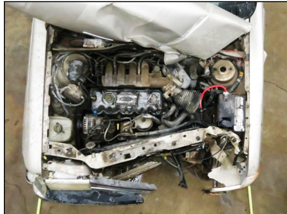
Figure 12: Deformation to the 1990 Ford Tempo's front plane from an overhead perspective.
