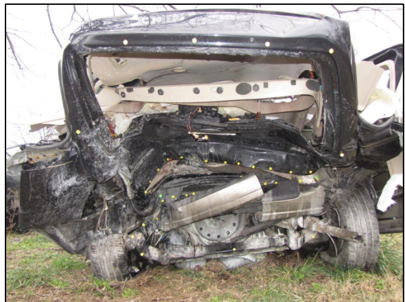
Figure 18: Image depicting the damage to the back plane of the Ford Windstar.
