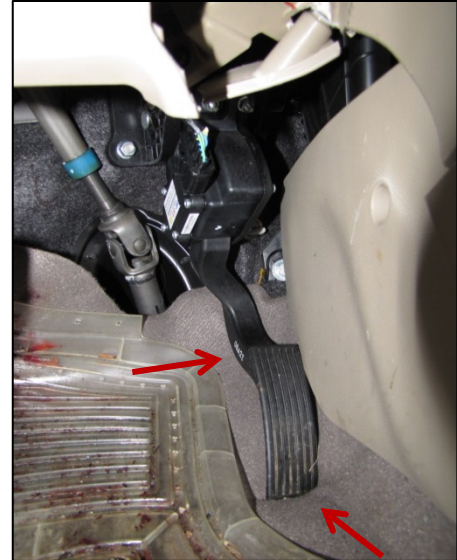
Figure 16: Image depicting the post-impact jammed accelerator pedal of the Kia.
