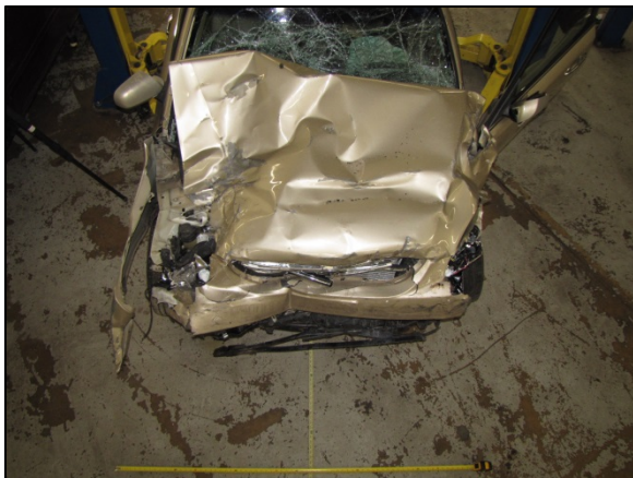
Figure 8: Overhead view depicting the frontal crush of the Kia. The horizontal tape measure represents the original length of the vehicle.
