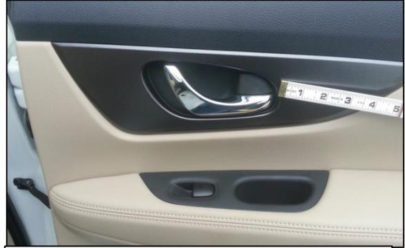
**Figure 5: Second row right door release lever and the rotating locking lever of an exemplar vehicle.**
