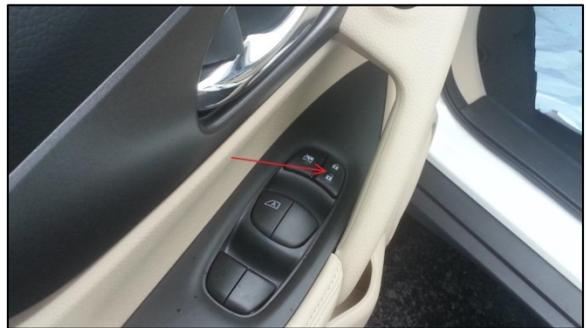
**Figure 6: Power locking rocker switch on the forward aspect of the driver's door panel.**
