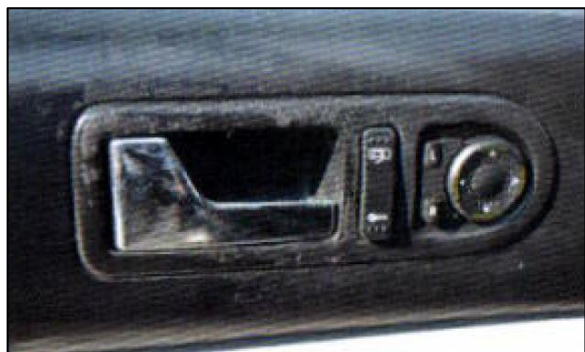
Figure 6. Driver side interior door lever of the involved 1998 Volkswagen Beetle. Image provided by the police agency.
