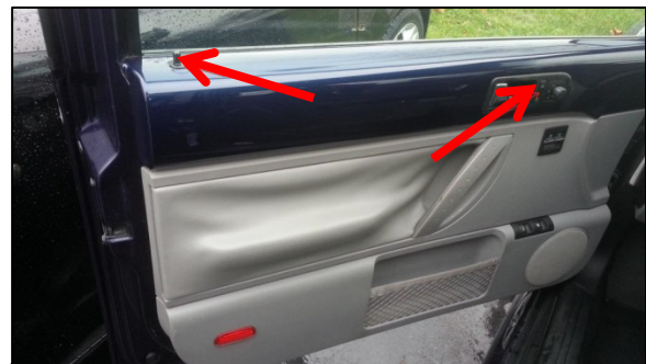
Figure 7. Locking modes (arrows) of an exemplar vehicle.
