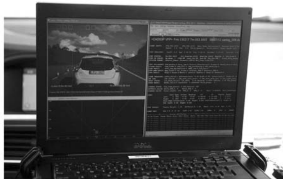
Test equipment for a Volvo prototype of autonomous driving support technology includes radar sensors and a camera to control speed, brakes, and steering to help a driver stay in the lane and follow traffic flow.
