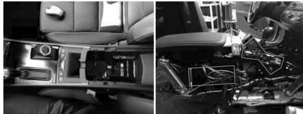
Figure 2. Fourth Generation touch-based sensor integrated in the DADSS X2 research vehicle center stack
