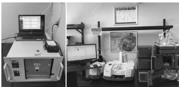
Figure 13. Thermo Fisher iS50 FTIR, Waters Aquity UPLC and MKS Multigas 2030 FTIR in the DADSS Research Laboratory
