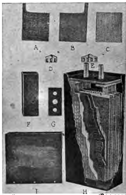
Fig. 35 Elements of Assembled Battery
