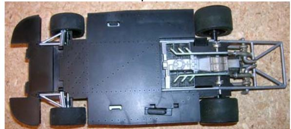
The wheels covers were painted black with gold spoke decals. The Dunlop lettering was also on the decal sheet. The wheels mount on metal axles, however the rear wheels needed several spacers to line up correctly as the gear that was to be used with the electric motor was not included. The front wheels mount with some pins from the outside, there are no pins for the back so I cut some large headed nails and glued them on to balance it out then, painted them all metallic grey.
