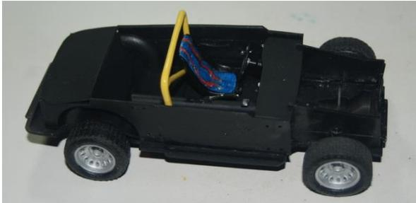
**Chassis:** There is one basic chassis pan, the interior is glued onto the upper side. Suspension detail is rather simple. The rear end and suspension is molded as one piece. The tires mount on a metal axle. The front A arms are molded to the frame, there are shocks which use a metal rivet to mount the tires.
