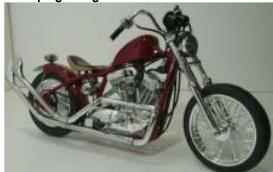
Body had the molded in turn signals and taillights removed, the toylike mirrors also removed and filled in. Painted in a rat rod/rust bucket style.
