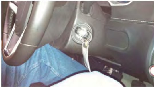
Camaro: Gen I flip key shown in RUN position, approximately 124 degrees CW from vertical.
