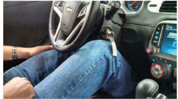
Camaro: 6' 3" occupant, foot on brake pedal, knee to key distance = 30 mm
