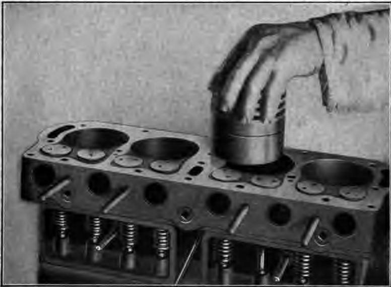
Fig. 72.—How Ford Piston May Be Withdrawn Through Top of Motor.
