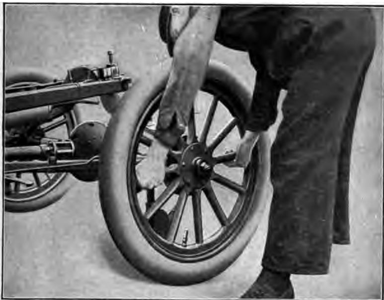
Fig. 64.—Method of Testing Rear Wheel Brakes, Also Wear in Axle Bearings.
