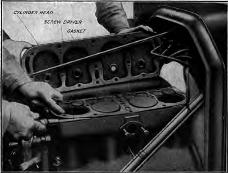
Fig. 69.—Showing Method of Removing Copper Asbestos Gasket Used Between Cylinder Head and Cylinder Block Casting of the Ford Engine.
