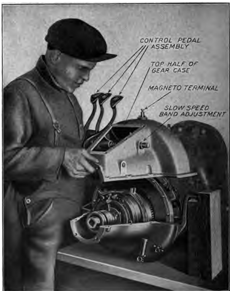
Fig. 90.—Showing How Transmission Cover is Removed to Permit Reaching Transmission Brake Bands.
