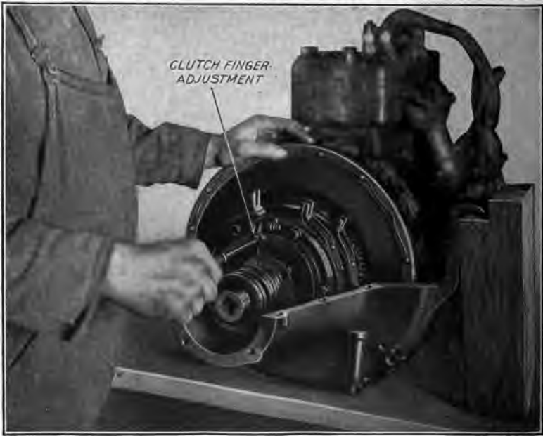
Fig. 61.—How to Tighten Slipping High Speed Clutch.
