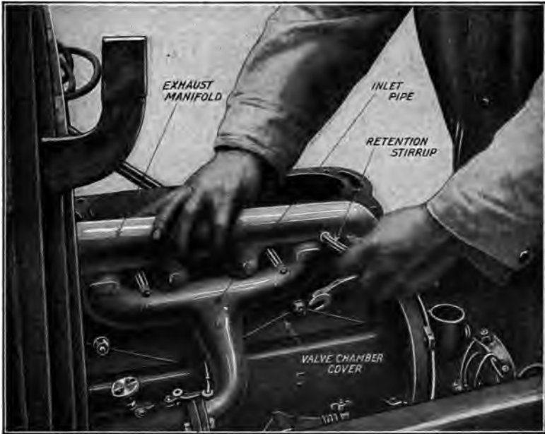
Fig. 70.—Method of Removing Inlet and Exhaust Manifold.
