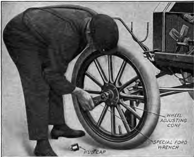
Fig. 63.—Showing Use of Special Ford Wrench in Adjusting Front Wheel Bearings.
