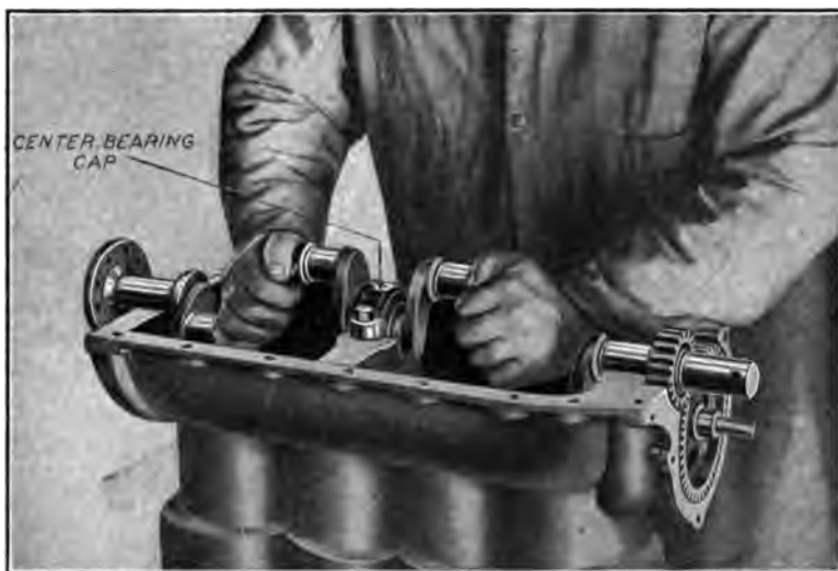
Fig. 80.—Showing Method of Testing Main Bearings When Refitting by Rocking the Crank Shaft by Hand.
