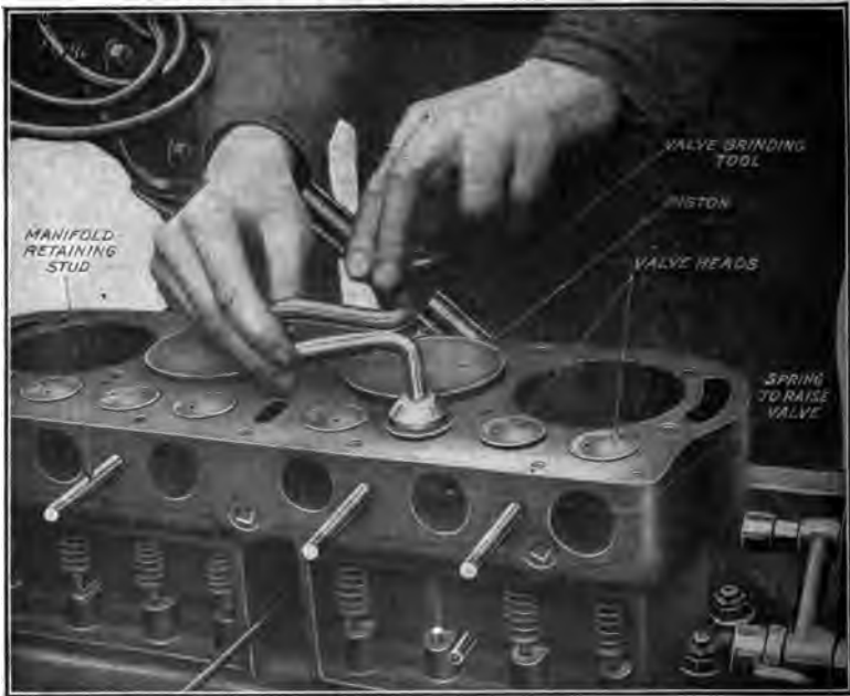
Fig. 78.—Showing Use of Special Tool for Grinding Ford Valves.
