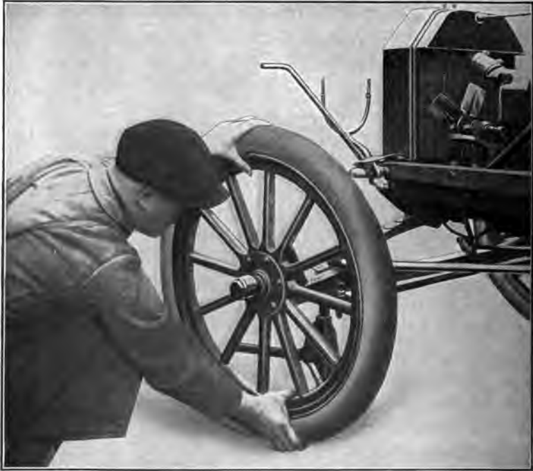
Fig. 62.—Testing for Front Wheel Looseness.
