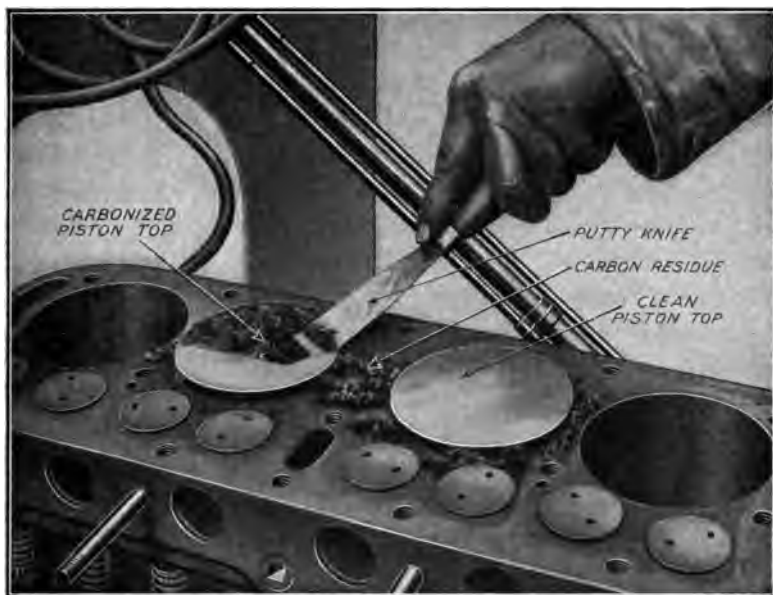
Fig. 74.—Method of Removing Carbon Deposits from Piston Top and Cylinder Block.
