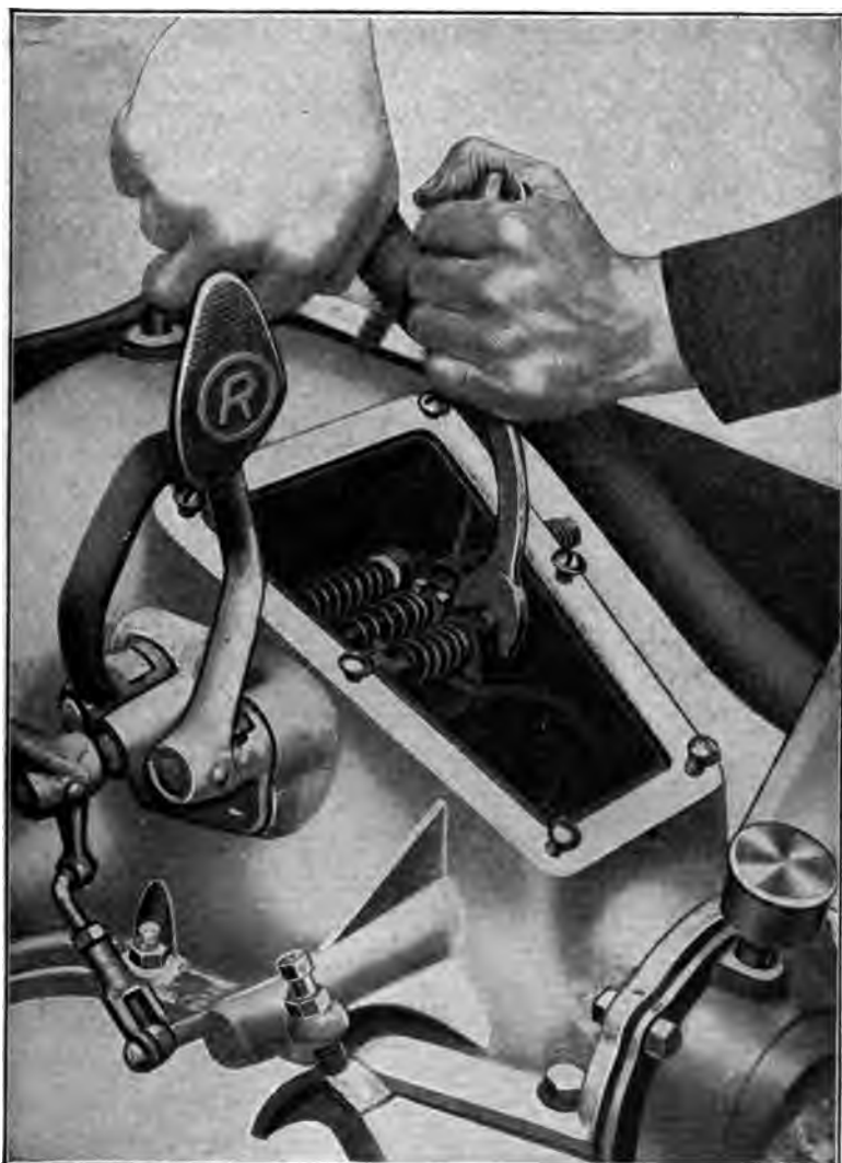
Fig. 60.—Method of Adjusting Transmission Brake Band.
