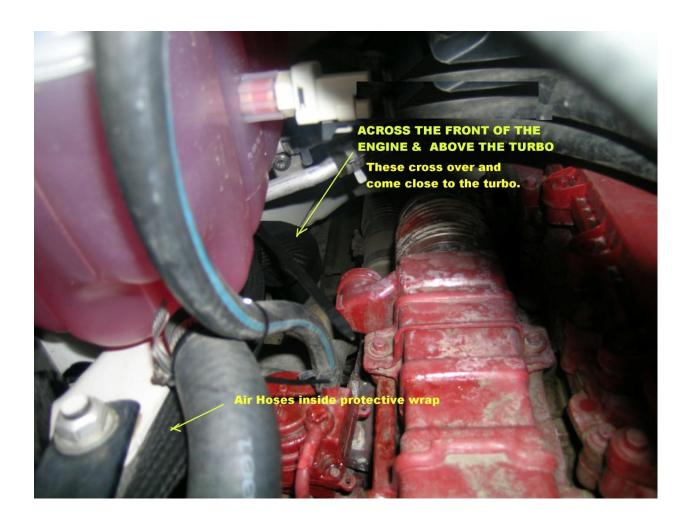
V. Identify the Remedy: The remedy for any melted air hoses is to remove the affected hoses, contact Fontaine Modification for parts, and replace with new hoses and thermal wrap as shown below. For Air Hoses that are improperly routed, the remedy is to route per the
