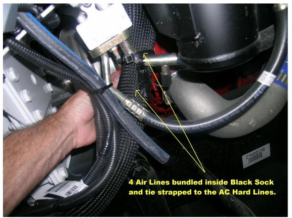
REMOVE RH SIDE FENDER TO GAIN ACCESS TO THE AIR LINES. SOCK MAY BE SILVER OR BLACK.
