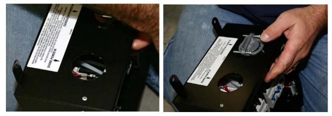
11. Using the original (4) screws, install the new transfer switch so that the shore line and generator inputs point toward the outside wall of the motorhome. NOTE: The original switch was mounted with wire entry from the bottom side. The new transfer switch must be installed so that wire entry is from the sides of the box. Power cables may need to be relocated to make room for the new switch.
