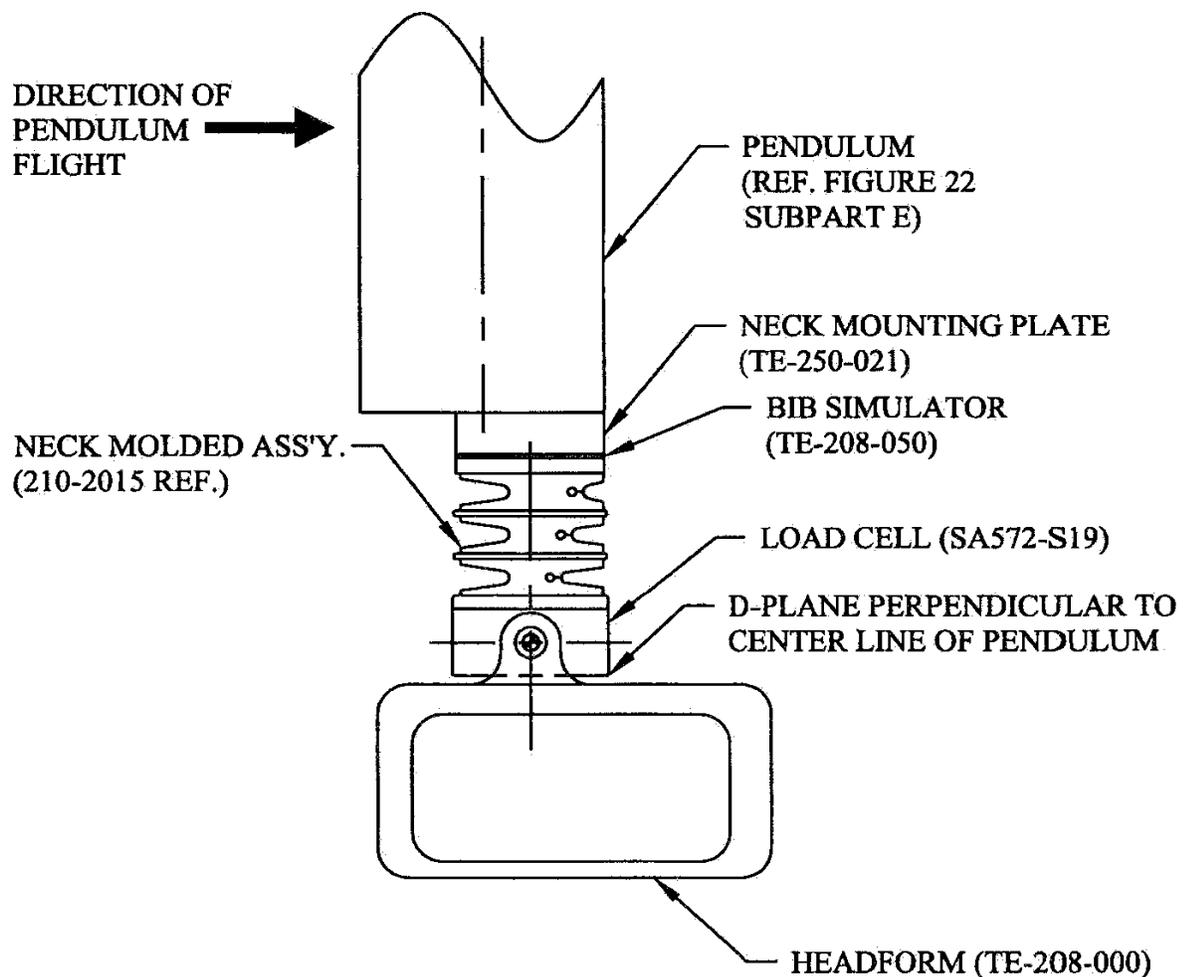
NOTE: MOUNT NECK AT LEADING EDGE OF PENDULUM TO AVOID INTERFERENCE WITH HEADFORM MOTION.
