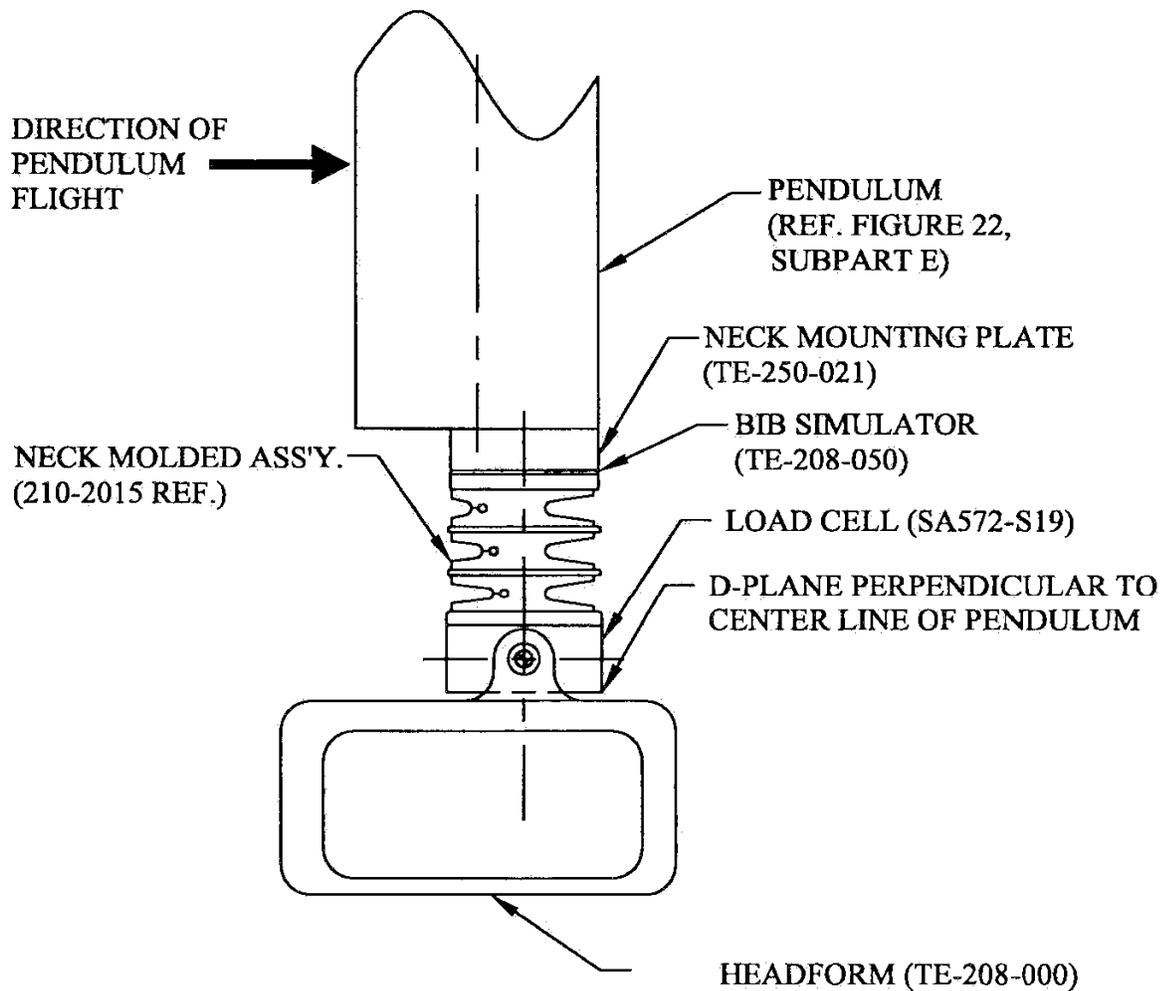
NOTE: MOUNT NECK AT LEADING EDGE OF PENDULUM TO AVOID INTERFERENCE WITH HEADFORM MOTION.
