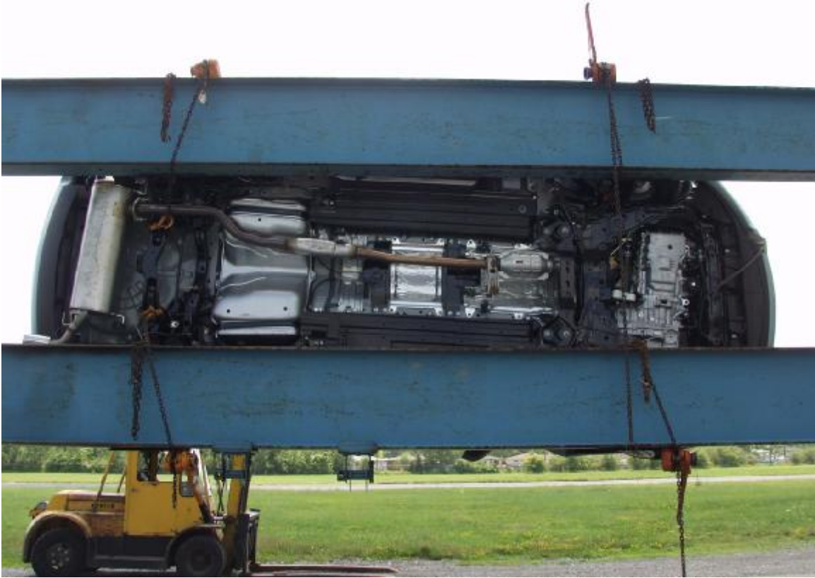
Figure A-51: Rollover 90 Degrees
