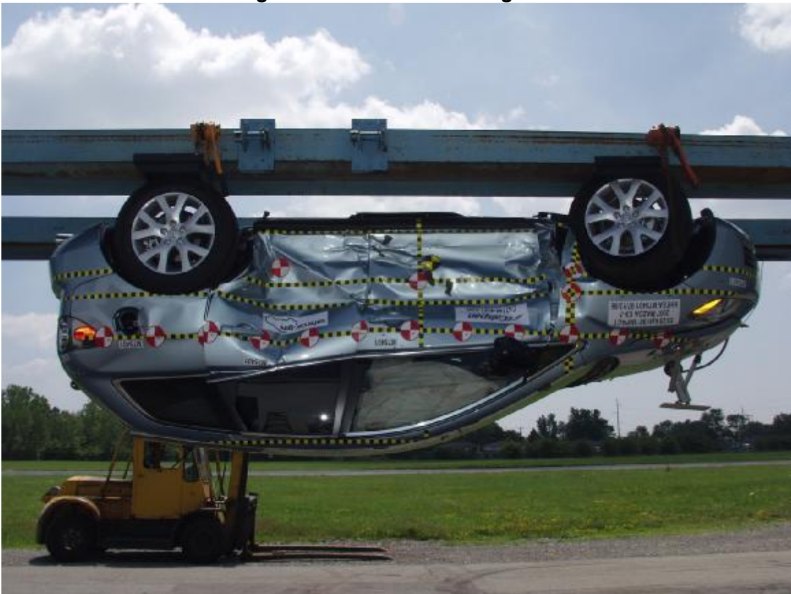
Figure A-52: Rollover 180 Degrees
