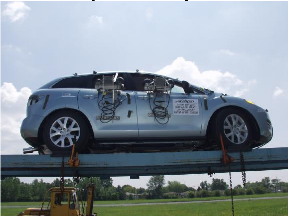
Figure A-54: Rollover 360 Degrees
