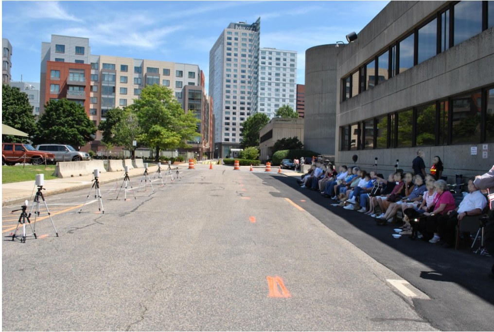
Figure 48. A Line of six Tripod-Mounted Loudspeakers was Positioned 25 Feet in Front of the Line of Participants to Present the Idle, Start-Up and Acceleration-From-Stop Sounds
