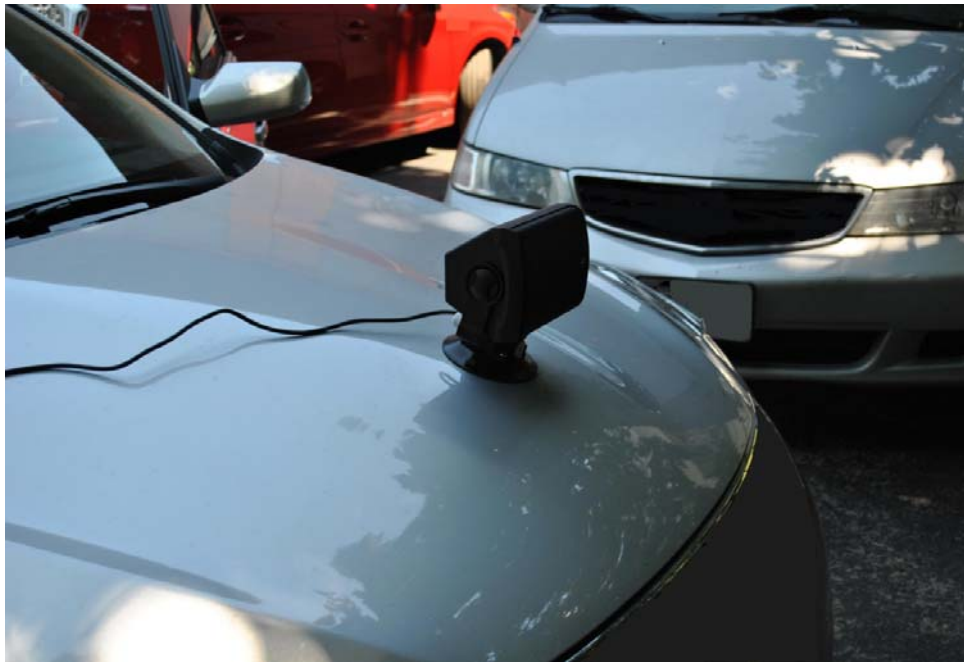
Figure 47. HEV Fitted With a Loudspeaker Temporarily Mounted on the Hood
