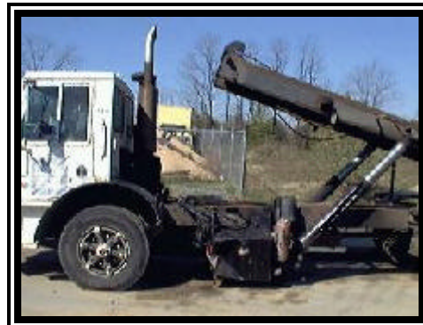
Figure 4. Impact damage to the (left side surface) hydraulic box of the 1982 Crane roll-off truck.
