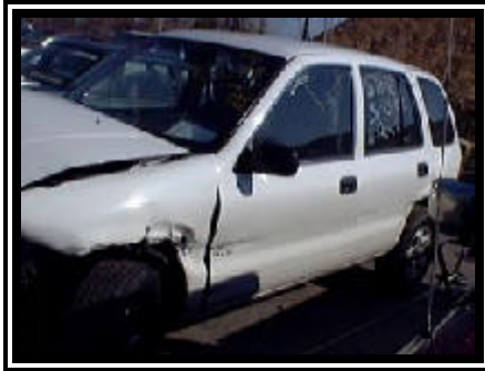
Figure 5. W-beam guardrail damage to the left side surface.
