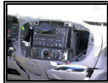
Figure 14. Center instrument panel showing separated panel
