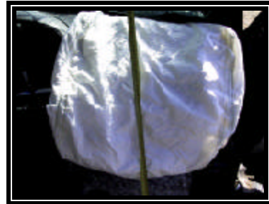
Figure 13. Redesigned front right passenger's air bag
