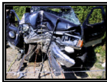
Figure 6. Damage to the Ford F150 pickup truck
