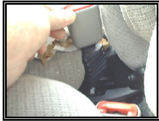
Figure 8: Right buckle and reportedly non-fired pretensioner.
