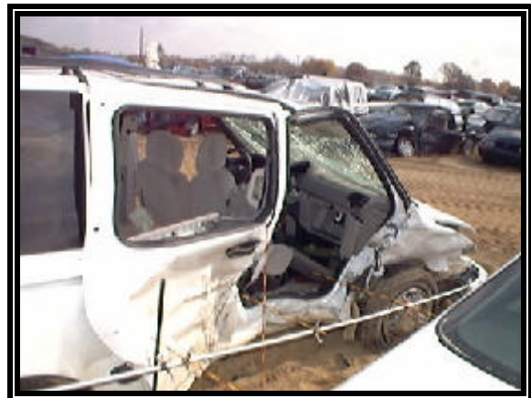
Figure 4: View of the right side damage to the Chevrolet Venture.
