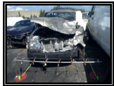
Figure 4. Frontal damage to the Kia Sportage
