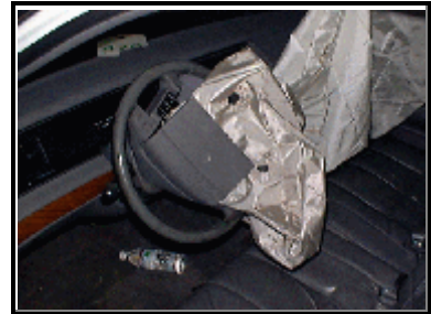
Figure 8. Overall view of the driver air bag, cover flaps, and the vent ports.
