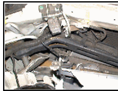
Figure 5. Overhead view of the crush profile to the cross member.
