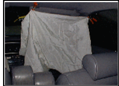
Figure 11. Deployment path of the front right air bag.
