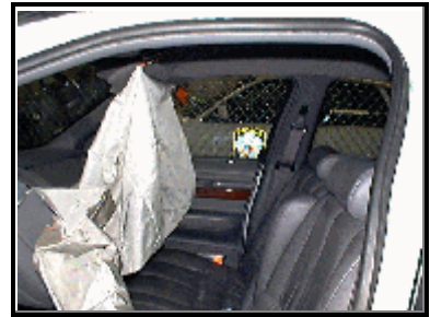
Figure 10. Profile view of the deployed front right air bag.
