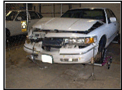
Figure 1. Frontal damage to the 1993 Grand Marquis.
