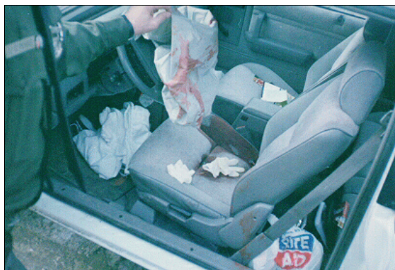
Figure 16: On-scene view showing case vehicle's deployed, blood stained, air bag and front seat positions prior to removal of air bag by family; Note: driver's seat was located at its forward-most position (case photo #47)
