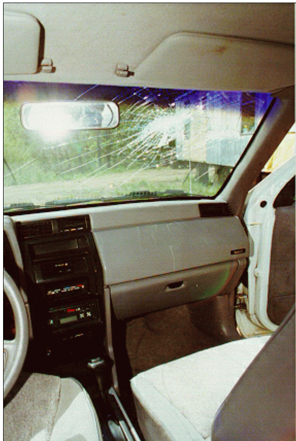
Figure 10: Vertical view of case vehicle's front right passenger seating area showing head contact to right windshield (case photo #24)
