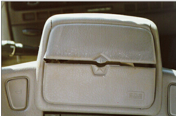
Figure 13: Close-up of suspected cloth transfer on case vehicle driver air bag module's top cover flap (case photo #28)
