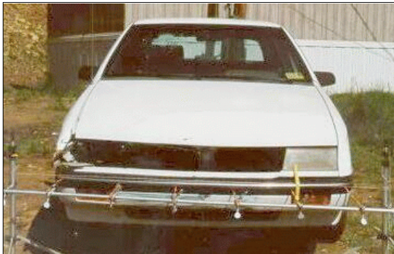
Figure 3: Case vehicle's front oblique damage; Note: yellow tape marks width (leftmost) of direct damage from Chevrolet (case photo #08)
