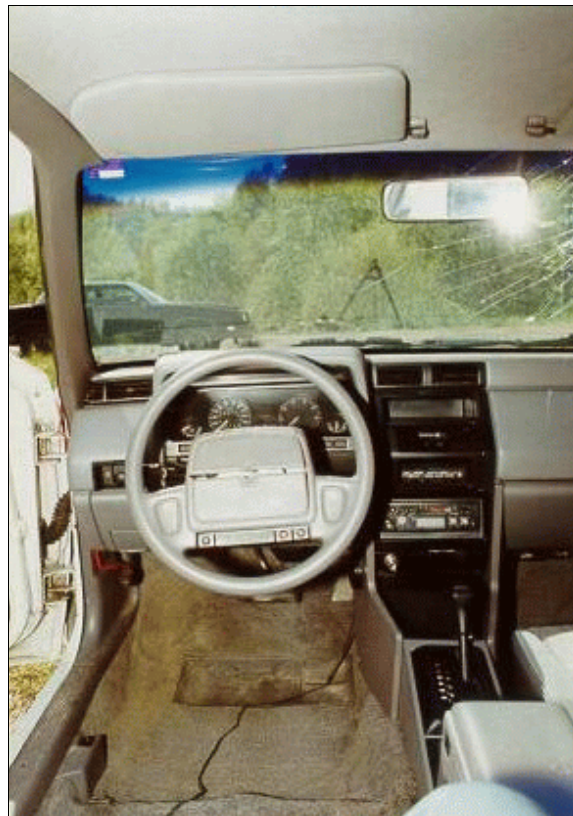
Figure 11: Case vehicle's driver seating area showing steering wheel, instrument panel, and greenhouse area with no apparent evidence of occupant contact; Note: air bag was cut out and driver's seat was removed by family (case photo #23)
