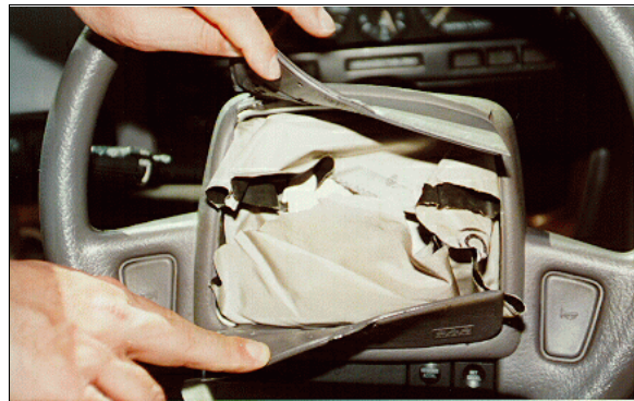
Figure 14: Close-up of interior of case vehicle's driver air bag module after air bag was cut out by family (case photo #29)
