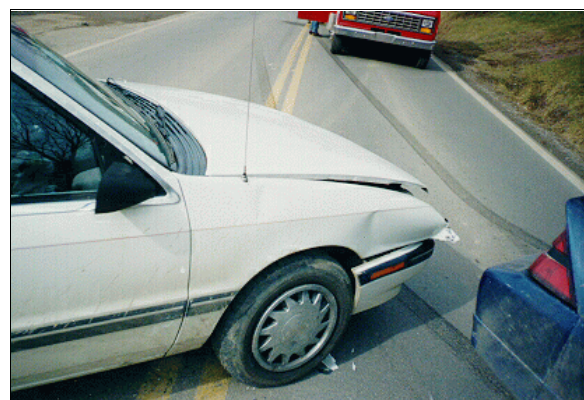
Figure 7: On-scene view looking north-northeastward showing case vehicle's final rest position straddling double yellow center lines and Chevrolet's evasive skid marks leading into case vehicle's front (case photo #46)
