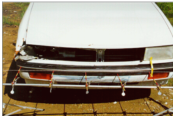
Figure 9: Elevated view of deformation to case vehicle's front with contour gauge present; Note: yellow tape indicates width (i.e., leftmost) of direct damage (case photo #09)
