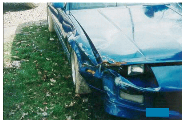
Figure 6: Attorney provided photo of Chevrolet's front right corner damage, viewed down right side from impact with case vehicle (case photo #42)
