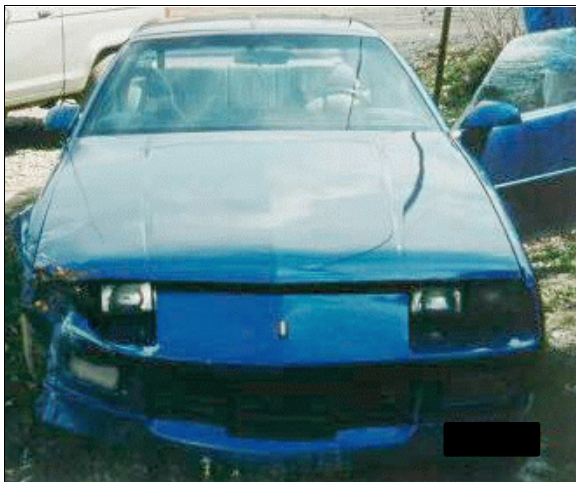
Figure 5: Attorney provided photo of Chevrolet's front right corner damage viewed from front at eye level (case photo #35)
