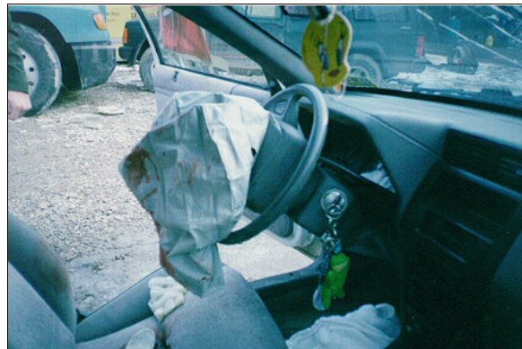
Figure 15: On-scene view of case vehicle's deployed driver air bag showing at least one vent port (case photo #49)
