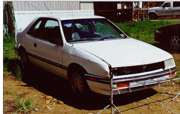
Figure 4: Case vehicle's frontal damage, viewed from right of front with contour gauge present, showing minimal deformation from oblique type impact with Chevrolet (case photo #16)
