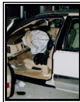
Figure 12. Police photo of vehicle interior with driver air bag and impeded deployment pattern.
