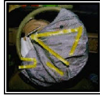
Figure 11. Contact evidence to the aft side of the air bag.
