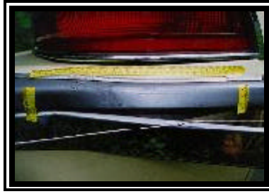
Figure 6. Right rear side surface damage.
