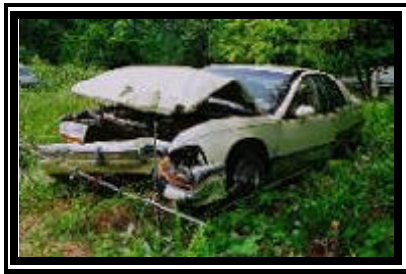
Figure 5. Frontal damage to the 1992 Buick Roadmaster Limited.
