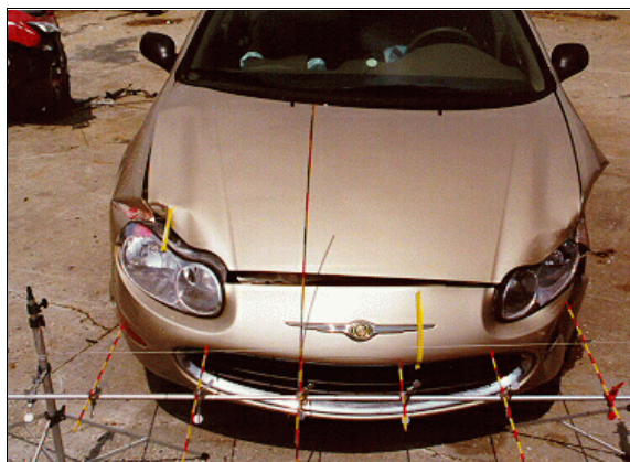
Figure 2: Elevated view of case vehicle's damaged front with tapes indicating start of direct damage; Note: tape at front right corner shows impact with straight truck while tape toward front left side shows impact with the Ford (case photo #15)
