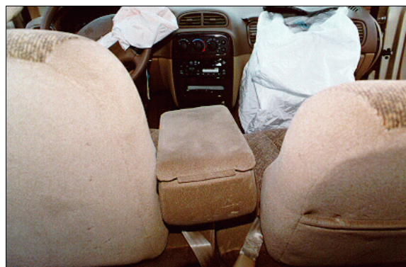
Figure 8: Case vehicle's damaged center arm rest which was bent towards driver's seat from contact by front right passenger's torso (case photo #39)
