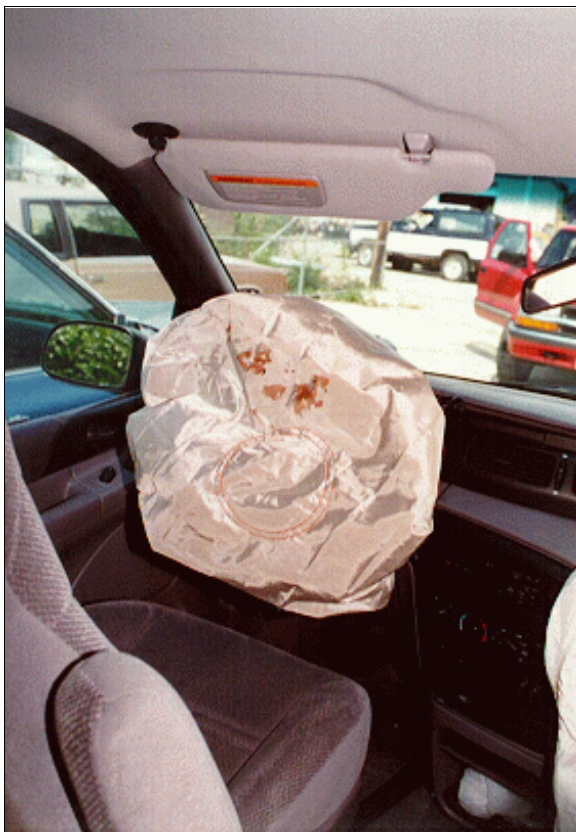
Figure 12: Vertical view of Ford's driver seating area showing deployed air bag with evidence (i.e., blood) of contact (case photo #75)
