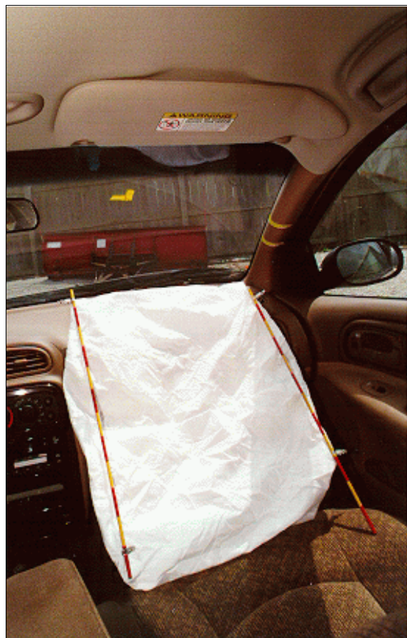
Figure 7: Vertical view of case vehicle's front right passenger seating area showing deployed air bag; Note: highlighted contacts on right "A"-pillar and scuff on windshield (case photo #40)
