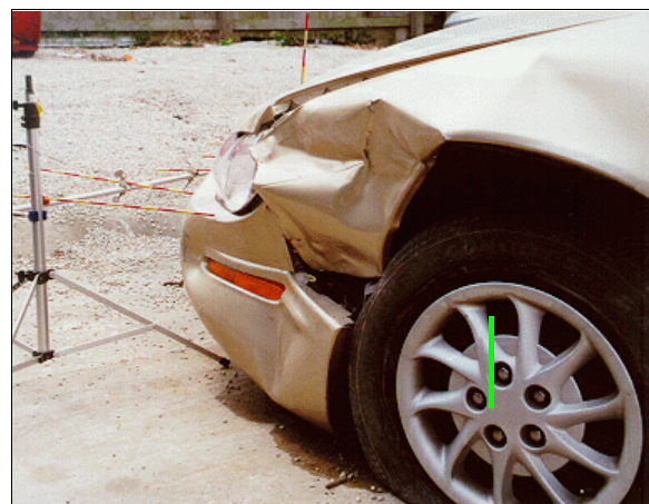
Figure 6: Case vehicle's left front corner showing direct damage extending back to hubcap of left front tire (case photo #25)
