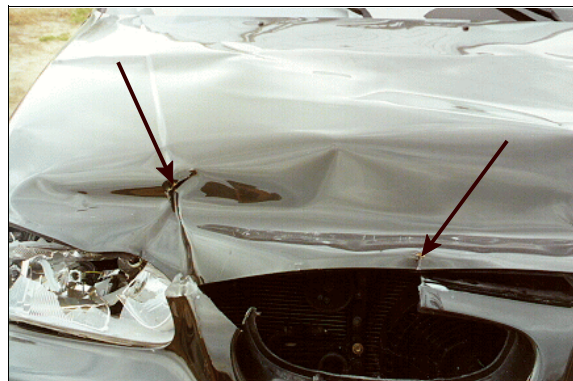
Figure 12: Close-up of creases in case vehicle’s hood from direct contact with Dodge’s tow hitch (case photo #08)
