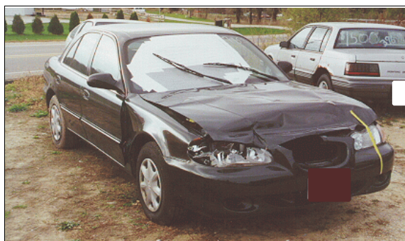
Figure 11: Case vehicle's frontal damage as a result of underriding Dodge; direct damage begins at front right corner and extends to yellow tape; Note: bent hood has been flattened out and right windshield wiper is bent outward at approximately its lower one-third from contact to windshield's glazing by front right passenger's head (case photo #19)
