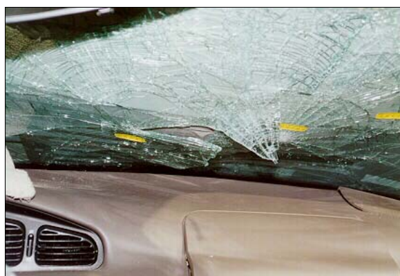
Figure 13: Close-up of case vehicle’s lower right windshield showing cracked and holed glazing from contact by front right passenger’s head and lower portion of right windshield wiper, respectively (case photo #28)
