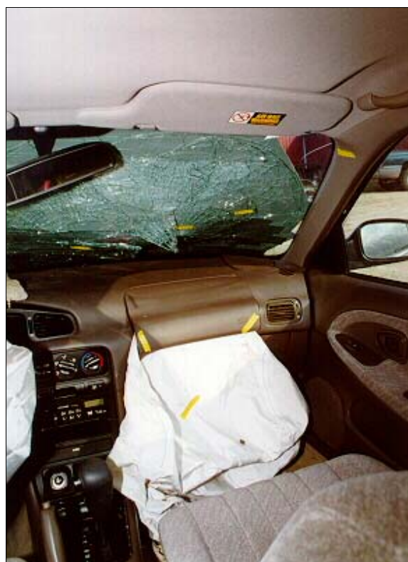
Figure 14: Vertical view of case vehicle’s front right passenger seating area showing contacted (tape) windshield, right “A”-pillar, front right air bag module’s cover flap and top of air bag (case photo #26)
