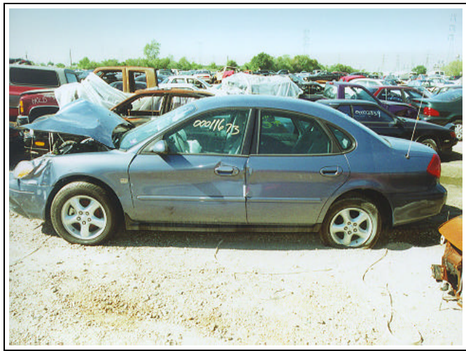
Figure 3. Left side damage to the case vehicle.
