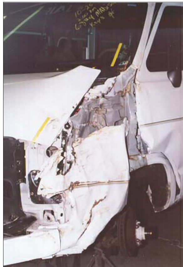
Figure 6: Close-up of case vehicle's narrow front left corner engagement with tree; Note: missing left front wheel and width (i.e., yellow tape) of direct damage (case photo #27)
