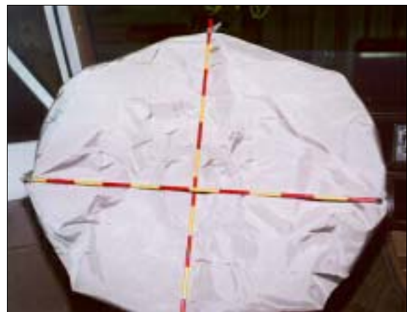
Figure 8: Case vehicle's deployed driver air bag; Note: no evidence of driver contact is visible (case photo #56)
