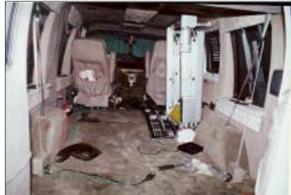
Figure 15: Case vehicle's interior "cargo area" viewed from back showing wheelchair lift and powered right side doors (case photo #59)
