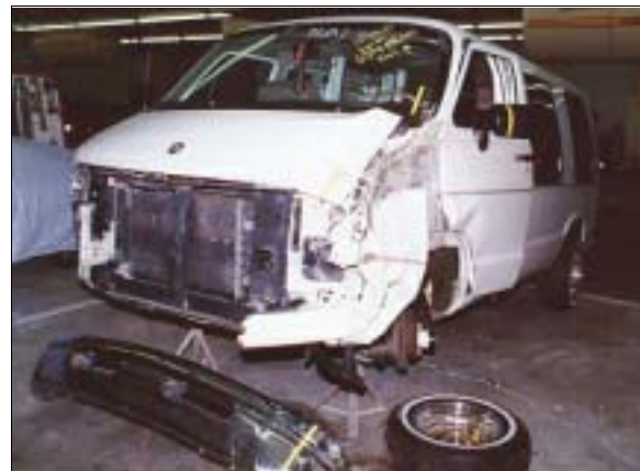
Figure 3: Case vehicle's damaged front left corner viewed from left of front showing narrow corner damage extending down left side; Note: direct contact to left windshield, "A"-pillar, and outside mirror (case photo #26)
