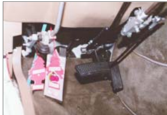
Figure 10: Close-up from left of center of case vehicle’s adaptive equipped control linkages for parking brake and brake and throttle controls (case photo #41)
