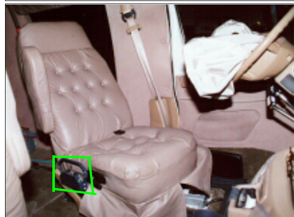
Figure 12: Case vehicle’s driver seat showing seat’s six-way powered hand controls (highlighted) along right side of seat; Note: deployed driver’s air bag and three-point safety belt system (case photo #47)
