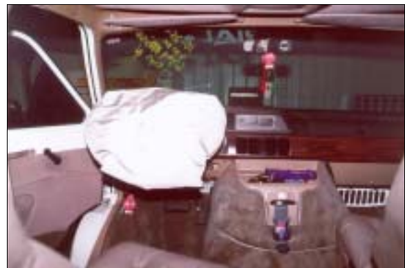
Figure 7: Case vehicle's front seating area, greenhouse, interior surface of driver's door, and deployed driver's air bag showing no obvious evidence of occupant contact (case photo #43)
