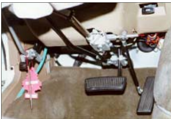
Figure 11: Close-up from right of center of case vehicle’s adaptive equipped hand control linkages for parking brake and brake and throttle controls (case photo #42)
