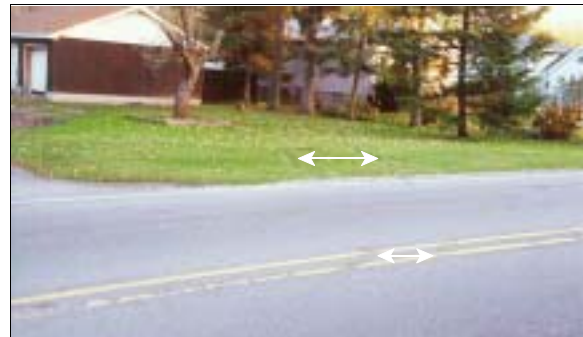
Figure 2: Case vehicle's transverse travel path across road from west shoulder area onto residential lawn and into tree; Note: arrows highlight tire scuffs (case photo #05)
