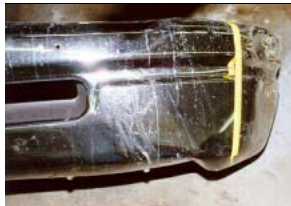
Figure 4: Close-up of direct contact (i.e., yellow tape outwards) to case vehicle's front left bumper corner from tree engagement (case photo #23)
