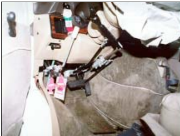
Figure 9: Case vehicle’s driver seating area viewed from driver’s door sill area showing vehicle’s adaptive equipped hand controls for parking brake and brake and throttle controls (case photo #39)
