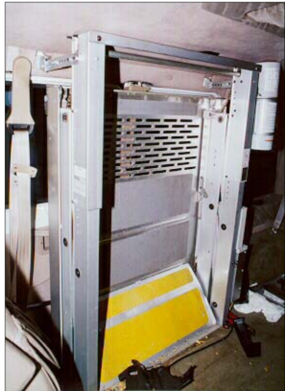
Figure 17: Close-up of case vehicle's powered wheelchair lift viewed from driver's seating area (case photo #62)
