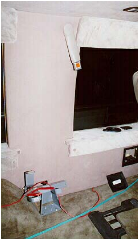
Figure 16: Case vehicle's floor mounted, wheelchair lock-down system located behind driver's seat and forward of left rear wheel well (case photo #60)
