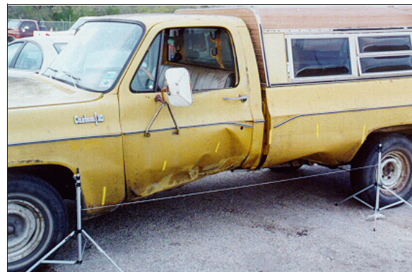
Figure 20: Chevrolet pickup's damaged left side with contour gauge present viewed from front of left (case photo #59)
