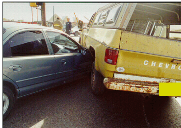
Figure 6: On-scene southeasterly view of case vehicle and Chevrolet pickup at final rest; Note: pickup tilted from being underridden by case vehicle (case photo #76)
