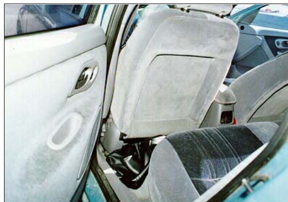
Figure 19: Back surface of case vehicle's driver seat back showing no visible evidence of contact on seat back (case photo #56)
