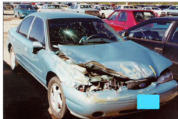
Figure 11: Case vehicle's front right deformation viewed from right of front; Note: underride type damage to hood and right fender (case photo #23)
