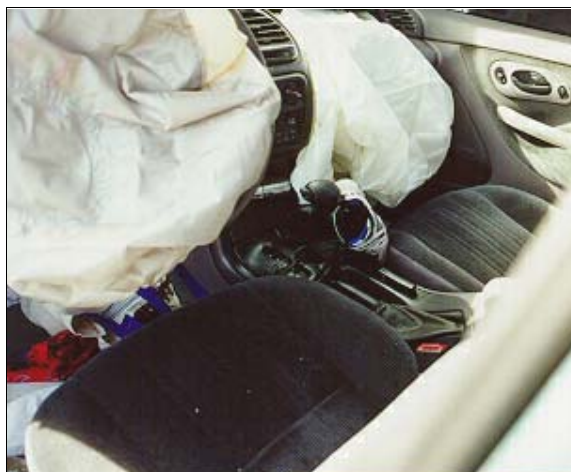
Figure 7: On-scene view of case vehicle's front seating area showing deployed air bags; Note: front right passenger's air bag was cutout and removed prior to inspection (case photo #80)
