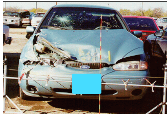
Figure 10: Case vehicle's frontal deformation with contour gauge present; Note: vertical yellow tape marks end of direct damage and damage is primarily above the bumper (case photo #13)
