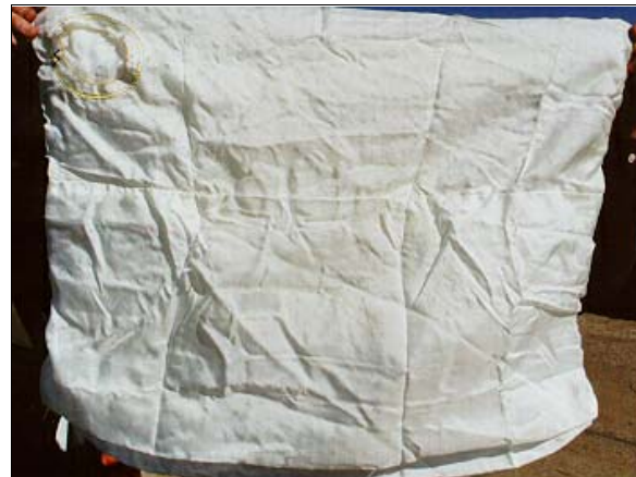
Figure 17: Frontal surface of case vehicle's front right passenger air bag showing no visible evidence of contact (case photo #44)
