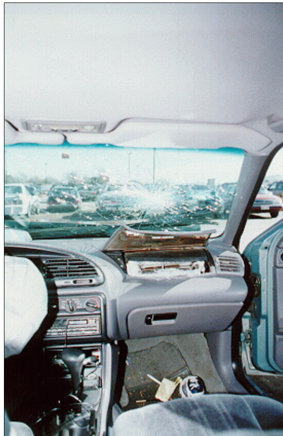
Figure 13: Case vehicle's front right seating area showing residue of deployed front right passenger air bag (cutout prior to inspection), air bag module's cover flap, spider web-type impact to right windshield's glazing, and blood spots on right roof (case photo #36)
