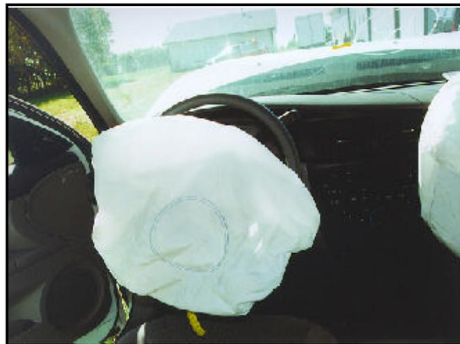
**Figure 3.** Case vehicle driver's air bag.
