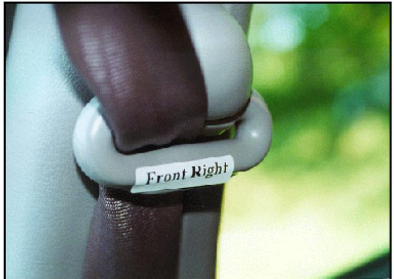
**Figure 12.** Belt loading marks—front right passenger
