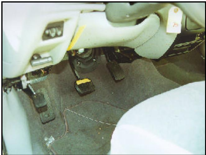
**Figure 5.** Case vehicle—damage to knee bolster cover and adjusted foot controls.
