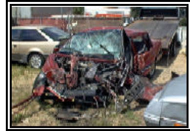
Figure 1. Overall view of the frontal damage to the Mercury Topaz.
