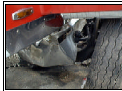
Figure 9. Deflected left corner of the front bumper.
