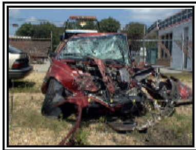
Figure 4. Frontal damage to the Topaz.
