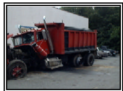
Figure 10. Fuel tank and tire/wheel damage.
