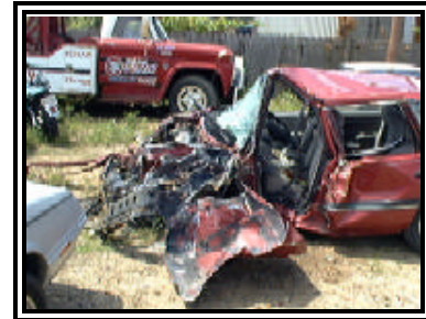
Figure 7. Compression of the frontal structure into the driver's compartment.
