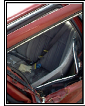
Figure 14. Left rear seated position and the belt loading evidence.
