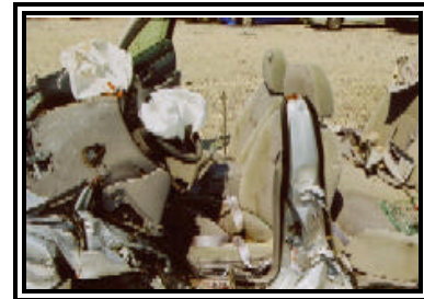
Figure 5. Intrusion into the driver’s position.
