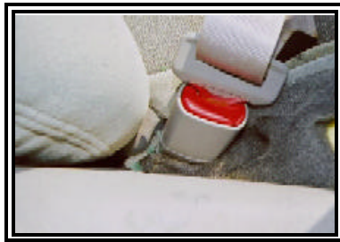
Figure 11. Fired driver's buckle pretensioner.
