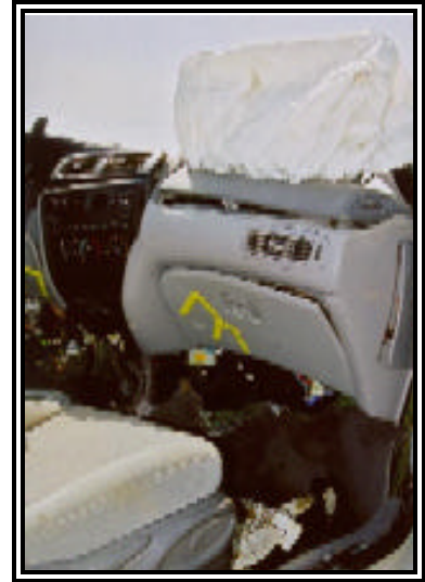
Figure 14. Front right passenger loading of the glove box and deployed air bag.
