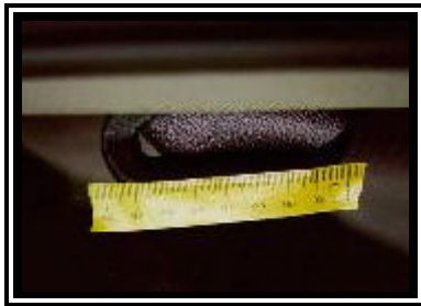
Figure 6. Abrasions to the front left restraint D-ring.
