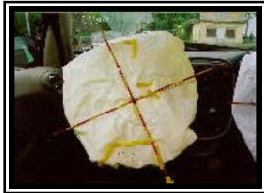
Figure 9. 2001 Chrysler PT Cruiser redesigned driver air bag.
