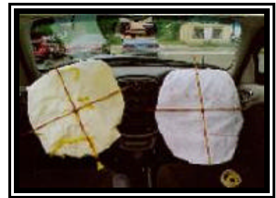
Figure 8. 2001 Chrysler PT Cruiser deployed redesigned frontal air bags.
