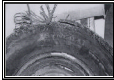
Figure 10. Closeup view of tire damage
