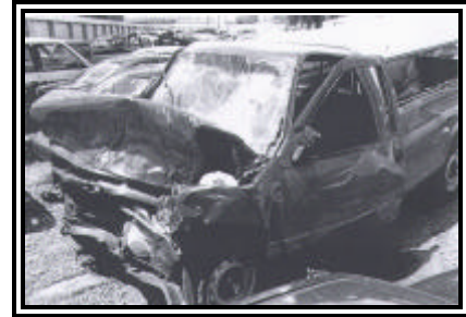
Figure 13. View of frontal damage to the 1992 Chevrolet pickup truck
