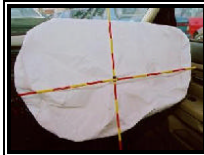
Figure 8. 2000 Ford Taurus LX deployed passenger air bag.
