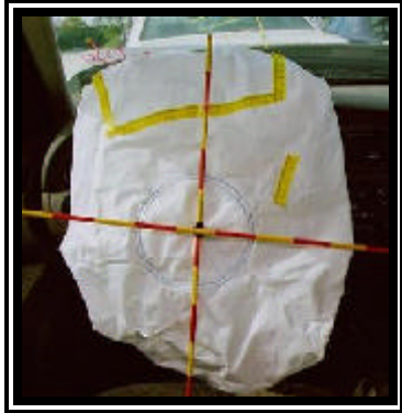
Figure 7. 2000 Ford Taurus LX deployed driver air bag.
