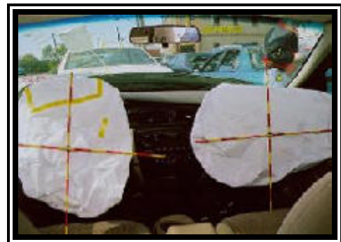
Figure 6. 2000 Ford Taurus LX deployed frontal air bags.
