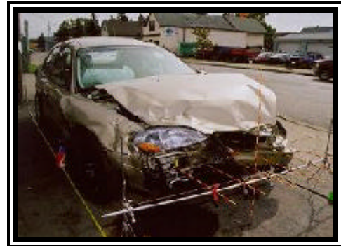
Figure 4. Front right damage to the 2000 Ford Taurus LX.
