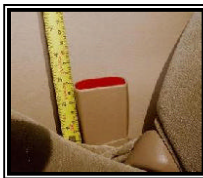
Figure 10. Driver restraint activated buckle pretensioner.
