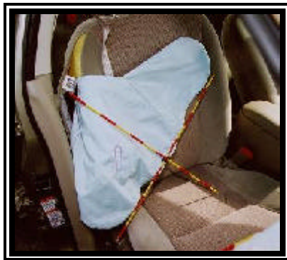
Figure 9. 2000 Ford Taurus LX deployed right front side impact air bag.
