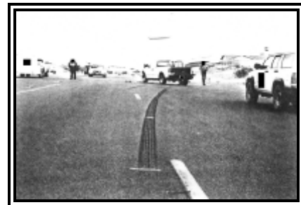
Figure 3. Northbound approach for the Ford pickup truck showing pre-impact skid marks
