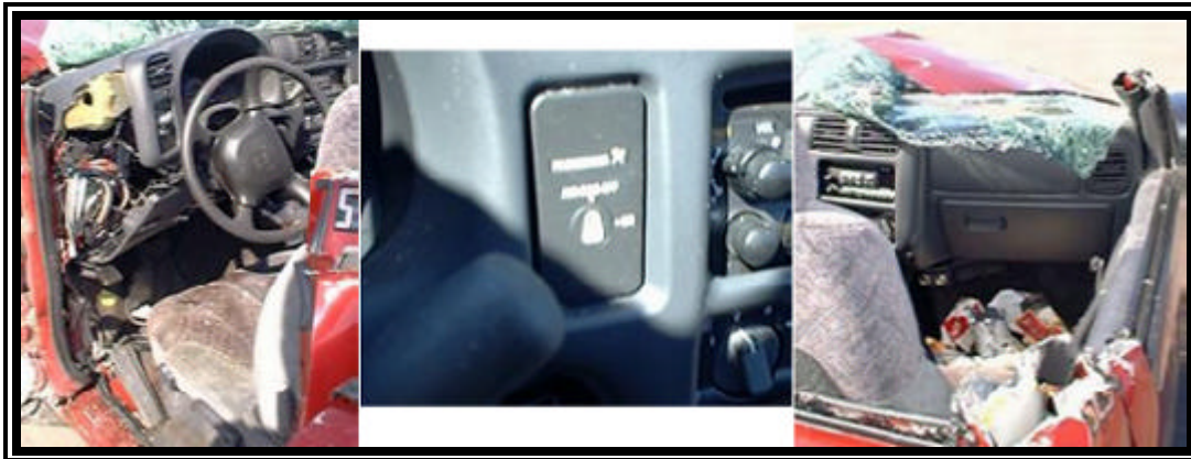
Figure 8. 2000 GMC Sonoma pickup truck non-deployed driver redesigned frontal air bag with the front right passenger air bag cutoff switch found in the “off” position.
