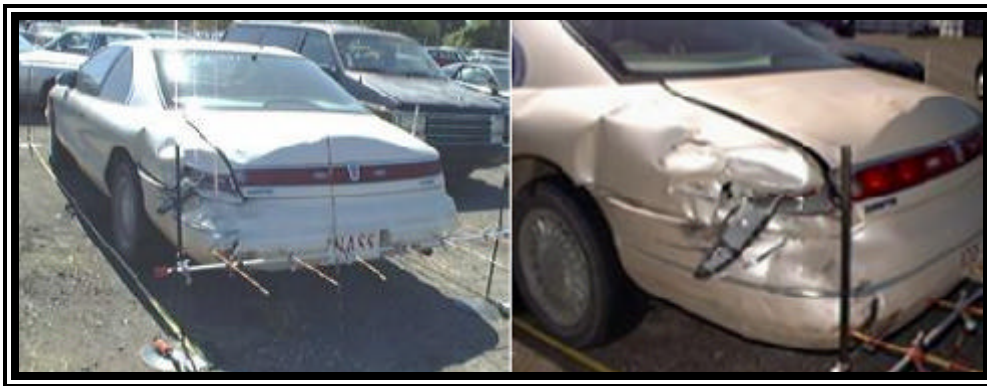
Figure 6. Impact #1 rear left damage to the 1995 Lincoln Mark VIII (V3).
