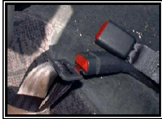
Figure 7. GMC driver manual restraint cut during post-impact driver extrication activities.
