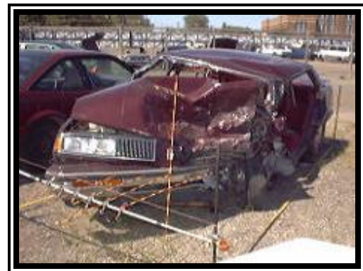
Figure 5. Impact #2 front left damage to the 1989 Oldsmobile Delta 88 Royale (V1).
