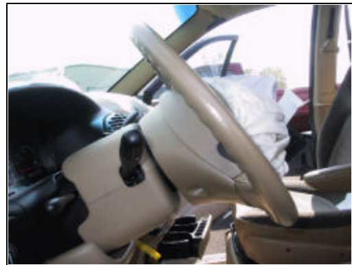
Figure 7. View of deformed steering wheel rim
