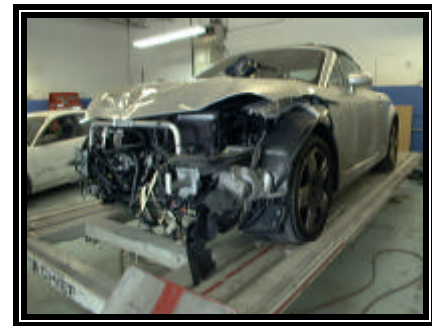
Figure 4. Frontal damage to the 2001 Audi TT
