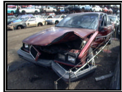
Figure 6. Left side damage from the primary impact and frontal damage from the breakaway sign post
