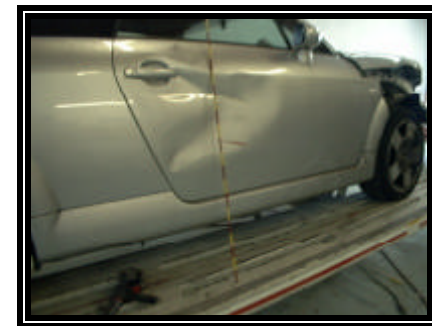
Figure 5. Right side sideslap damage to the 2001 Audi TT
