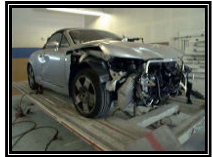
Figure 1. Front and side damage to the 2001 Audi TT
