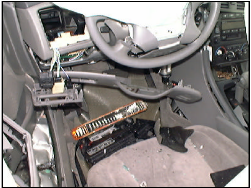
Figure 8. Lower steering wheel rim and knee bolster
