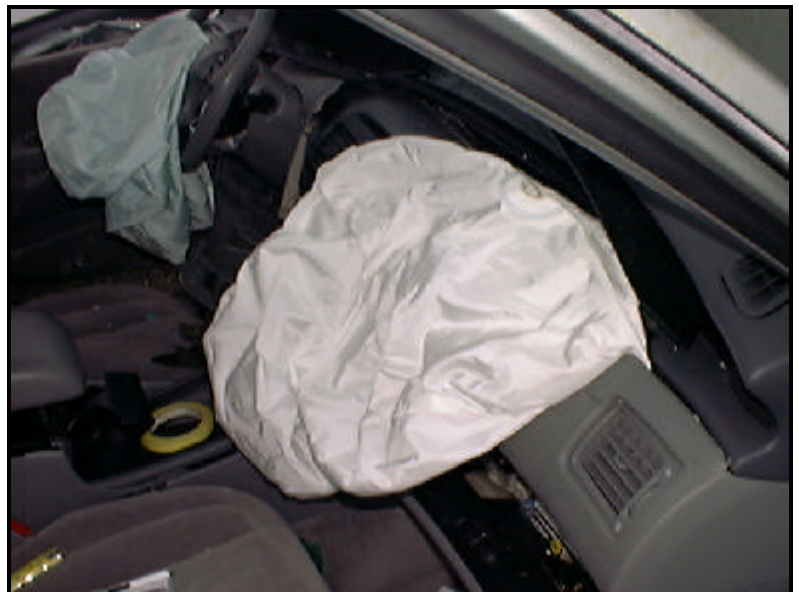
Figure 9. Frontal air bags/deformed steering wheel
