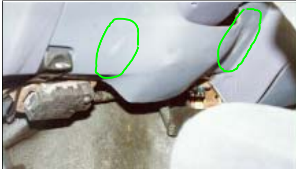
Figure 10: Knee contacts (highlighted) on case vehicle's driver knee bolster (case photo #23)
