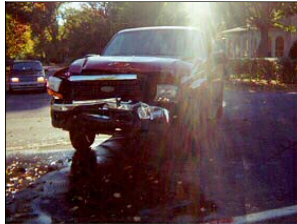
Figure 21: On-scene view looking east at Excursion's frontal damage; Note: Excursion's front has been shifted toward right (case photo #39a)
