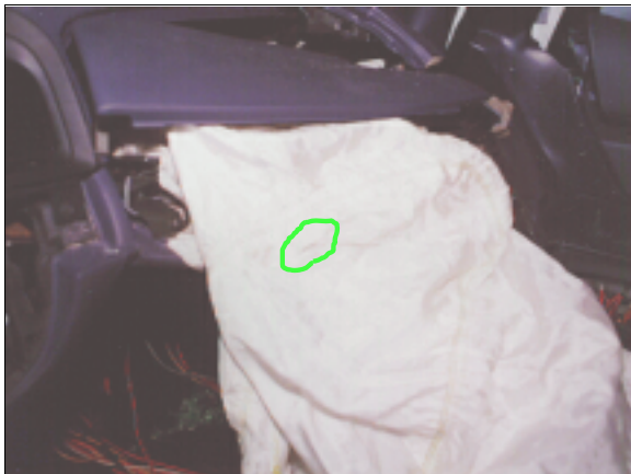
Figure 15: Case vehicle's front right passenger's air bag showing black scuff mark (highlighted) on right side of air bag from contact with black laptop computer or docking station (case photo #30a)
