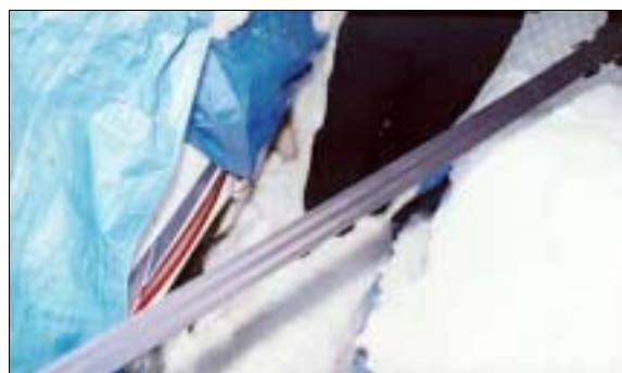
Figure 17: Webbing from case vehicle's driver safety belt system showing no visible evidence of loading or blood on webbing (case photo #31)
