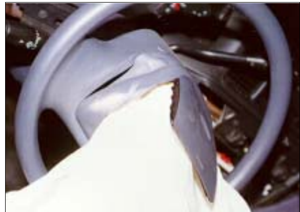
Figure 13: Close-up of case vehicle's steering wheel showing air bag module partially separated from hub during air bag's deployment (case photo #25)
