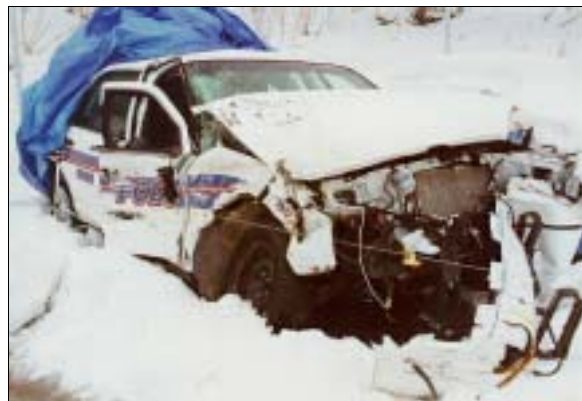
Figure 2: Case vehicle's damaged right front viewed from right of front which resulted from impact with Excursion's front; Note: frontal damage from tree impact (case photo #17)
