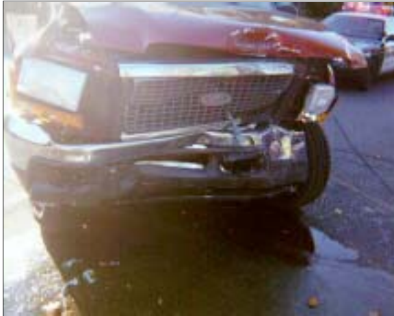
Figure 4: On-scene view looking southeast at Excursion’s frontal damage; Note: direct contact to front edge of hood from impacting case vehicle’s right “A”-pillar (case photo #39)
