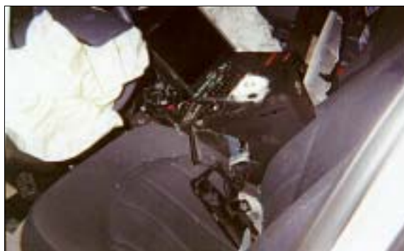
Figure 19: Post-crash view of case vehicle's front seating area showing damage to laptop computer and specially equipped center floor console (case photo #43)
