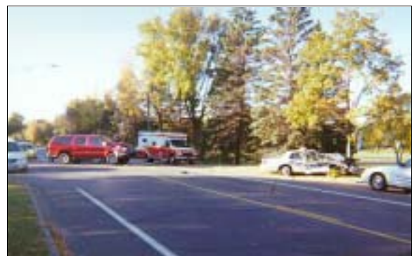
Figure 8: On-scene view looking in a south-southwesterly direction at final rest positions of the case vehicle—against a tree off the west side of the roadway, and the Excursion—straddling the northbound lane (case photo #40)
