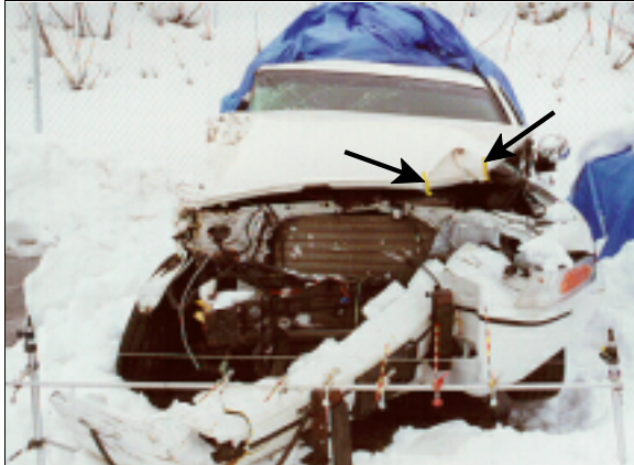
Figure 6: Case vehicle’s frontal deformation from both impacts; Note: tree impact (highlighted by yellow tape and arrows) and outward movement of front right bumper (case photo #09)
