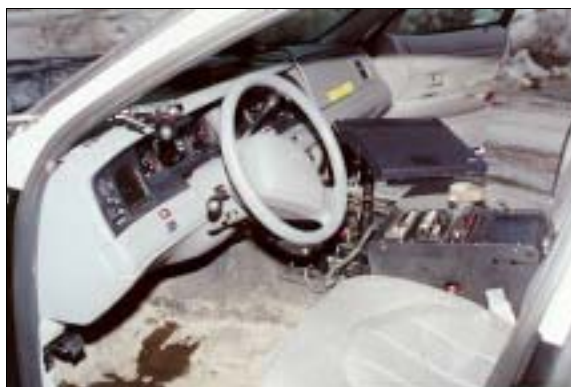
Figure 20: Interior view of an exemplar, undamaged Ford Crown Victoria, police vehicle showing laptop's position in docking station (case photo #47)
