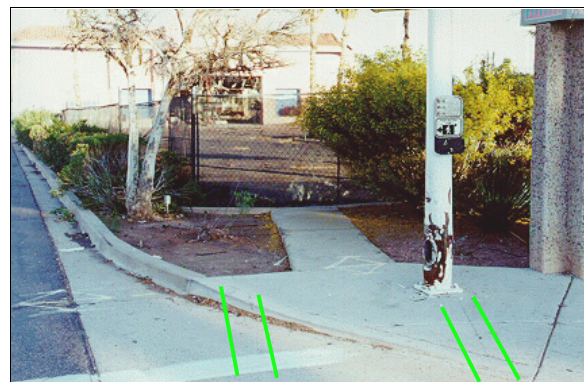
Figure 2: Case vehicle's east-southeastward travel path into southeast corner of intersection showing impacts with signal pole, small tree (torn away), and fence/fence post; Note: tire marks (highlighted) leading into signal pole (case photo #07)
