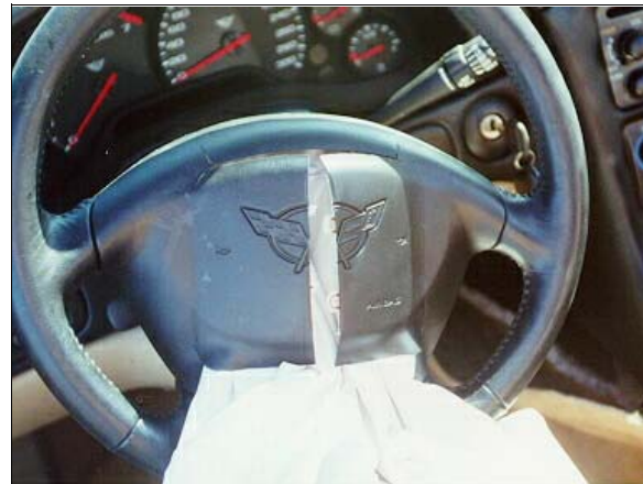
Figure 9: Close-up of case vehicle's driver air bag module showing deployed air bag and opened cover flaps (case photo #55)
