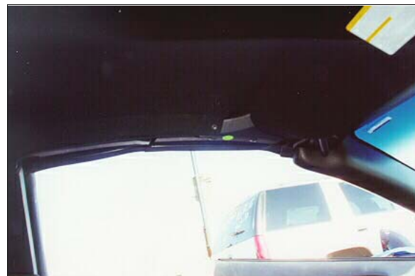
Figure 13: Interior view from right showing contact (i.e., dot) to case vehicle's left side roof rail by top of driver's head (case photo #49)
