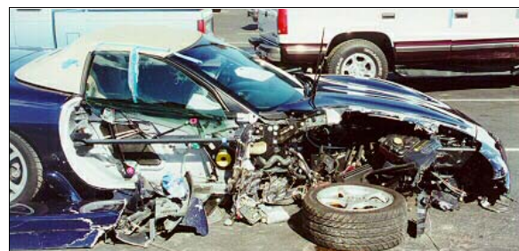
Figure 4: Case vehicle's right deformation; Note: right front door panel peeled away and right front tire assembly torn off (case photo #28)
