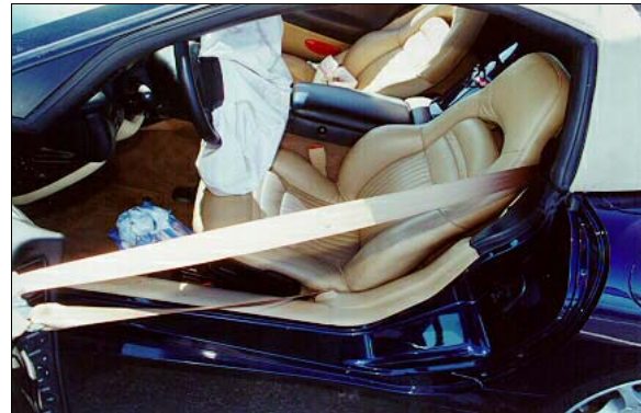
Figure 12: Case vehicle's driver seat belt webbing showing no evidence of usage during the crash (case photo #41)
