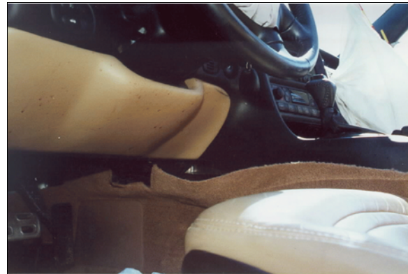
Figure 8: Knee bolster for case vehicle's driver showing probable knee contact on right side of steering column (case photo #40)
