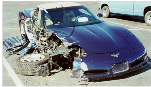
Figure 3: Deformation to case vehicle's front right showing damage extending down right side with right front tire torn off (case photo #33)
