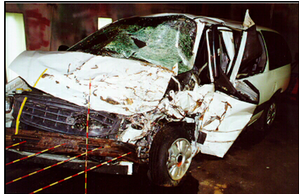
Figure 3: Case vehicle's front and left side damage (case photo #18)
