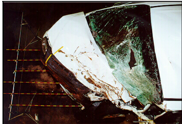
Figure 4: Overhead view of case vehicle's front end deformation (case photo #14)
