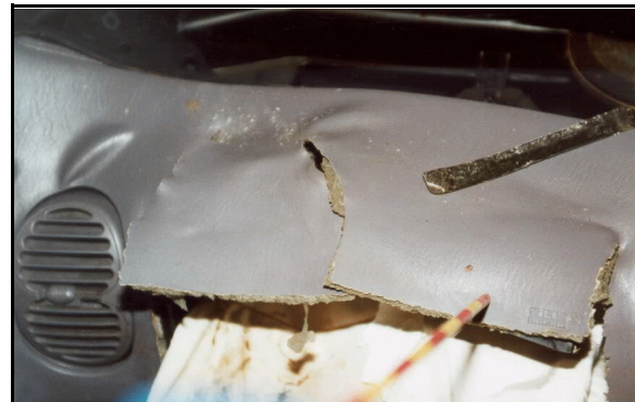
Figure 7: Front right passenger air bag module's torn upper cover flap (case photo #37)
