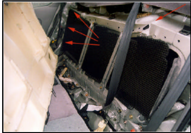
Figure 5. Damage to frame directly in front of traction battery.
