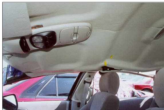
Figure 19: Case vehicle's right side roof rail and probable avenue of ejection for second seat passenger; Note: tape on roof indicates blood spots (case photo #30)
