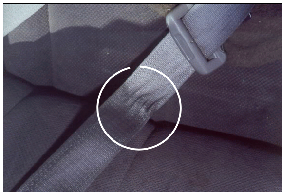
Figure 17: Close-up of loading evidence on webbing of case vehicle's second seat left passenger seat belt (case photo #45)
