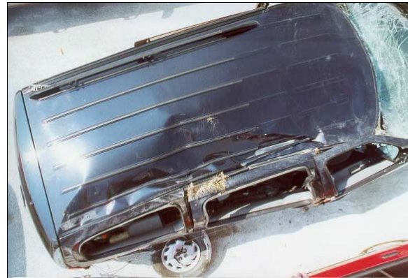
Figure 10: Overhead view of rollover damage to case vehicle's top and right side; Note: dis-integrated glazing on entire right side (case photo #25)
