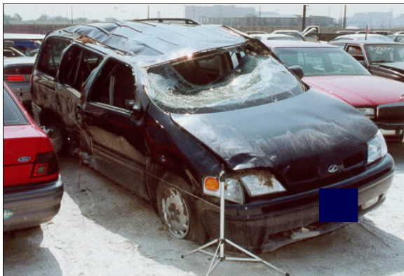
Figure 3: Case vehicle viewed from front right showing rollover and right side impact damage; Note: holed windshield (case photo #29)
