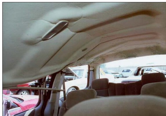
Figure 20: Right side of case vehicle's roof showing intrusion and probable avenue of ejection for back left seat passenger (case photo #48)
