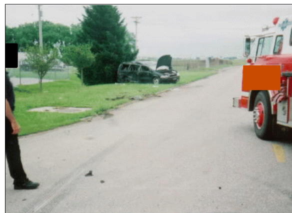
Figure 6: On-scene east-northeasterly view showing case vehicle's tire marks leading to rollover and final rest positions (case photo #66)
