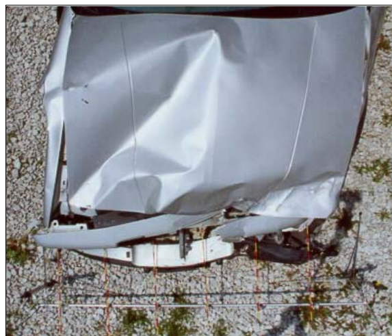
Figure 22: Overhead view of Buick's frontal deformation from impacting case vehicle's right side (case photo #52)
