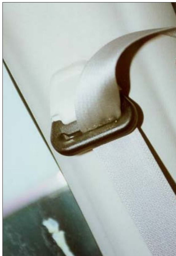
Figure 18: Close-up of "D"-ring for case vehicle's second seat left passenger showing friction rub and particles caused by loading (case photo #43)
