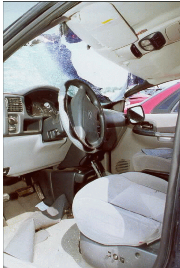
Figure 11: Vertical view of case vehicle's front seating area showing non-deployment of air bags; Note: driver's contact (yellow tape) to sun visor (case photo #31)
