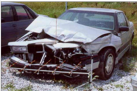
Figure 5: Frontal damage to Buick from impacting case vehicle's right side (case photo #57)
