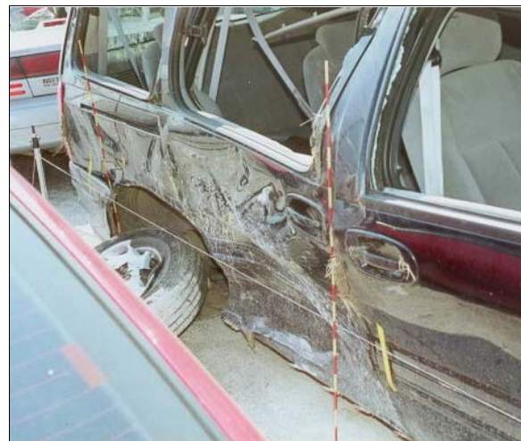
Figure 4 Close-up of case vehicle's right side damage from impact with Buick; Note: broken off right rear tire on ground (case photo #27)
