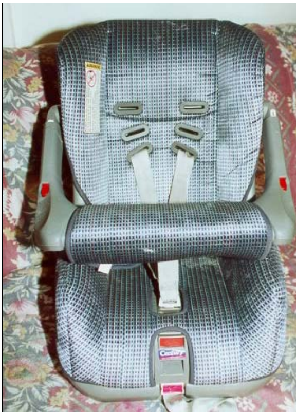
Figure 12: Convertible child safety seat used by case vehicle's second seat left passenger; Note: harness straps in bottom slots and should have been in top slots (case photo #61)
