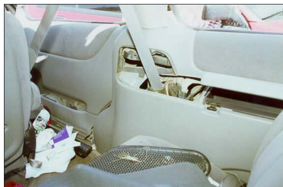
Figure 21: Case vehicle's right rear door and back seat interior panels showing absence of visible contact evidence during rollover and ejection by case vehicle's second and third seat passengers; Note: panel covering second seat's safety belt retractor has been knocked out (case photo #40)
