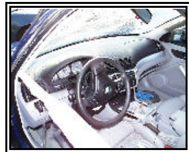
Figure 6. Non-deployed frontal air bags.
