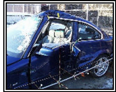
Figure 5. Left side damage from the pole impact.
