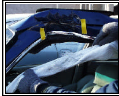
Figure 8. Deployed HPS with lacerations to membrane.
