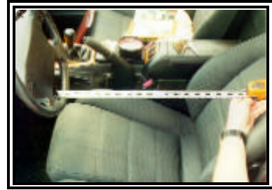
Figure 4. Profile view of the driver's compartment with the seat track adjusted to the full rear position.
